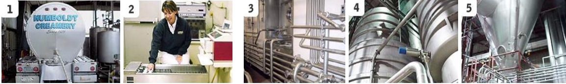
1) Milk arrives fresh everyday to be processed. 2) Each load of fresh milk is tested for quality and content. 3) Milk is pasteurized & separated into milk/cream. 4) Water is evap. off. 5) Milk is dried into Flakes or granules.
